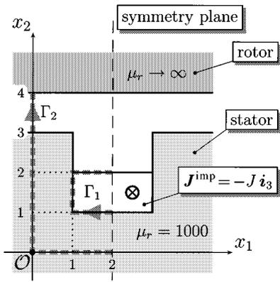
Fig. 1. Configuration concerning the test-slot problem  $J = 1 \text{ A} \cdot \text{m}^{-2}$ . Impressed boundary conditions  $\mathbf{n} \times \mathbf{H} = 0$  along  $x_1 = 2$  and  $x_2 = 4$  and  $\mathbf{n} \cdot \mathbf{B} = 0$  otherwise. Dimensions are in meters.
